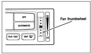
When you move the thumbwheel, the fan speed will go to manual control. The display window will show the symbol in the upper left corner along with the selected temperature and operating function.
